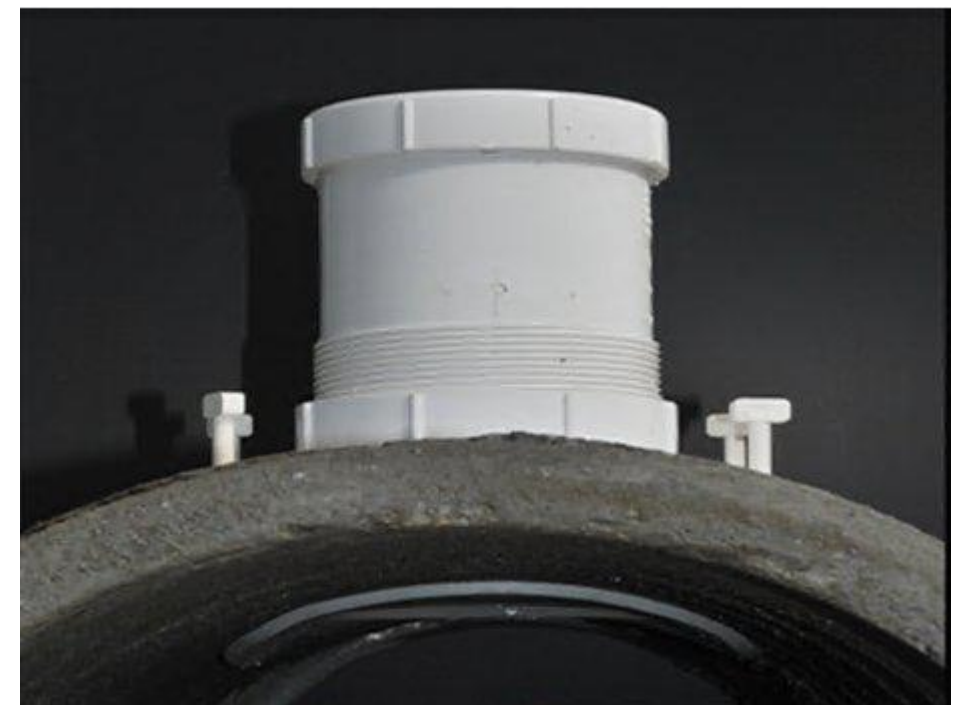
IMAGE: 'CONCONNECT' FITTING JOINED TO R.C.P. DRAINAGE LINE
